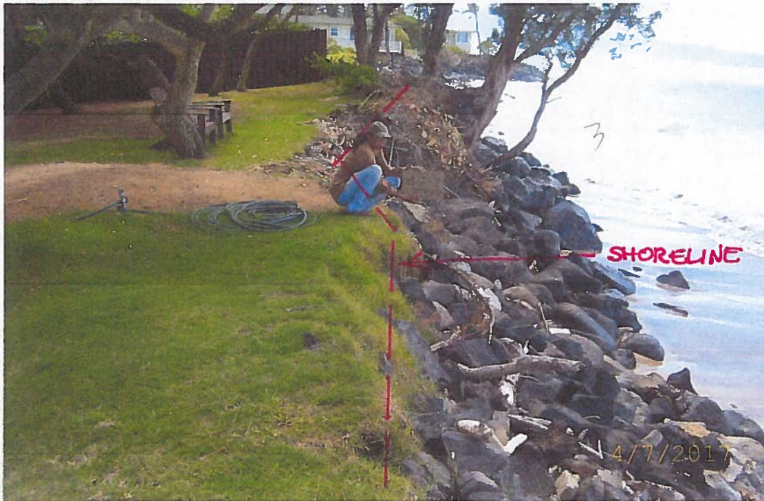
Photo No. 3: Taken from the east side looking westward. "Shoreline" follows top of bank approximately as marked.
